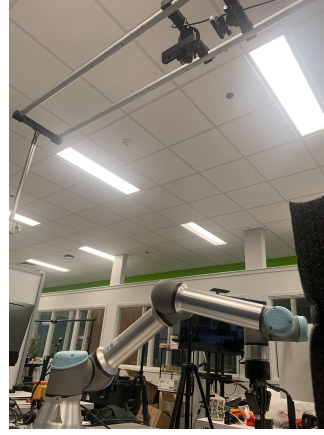
(b) Ceiling-mount stereo rig above the UR5e workspace.
